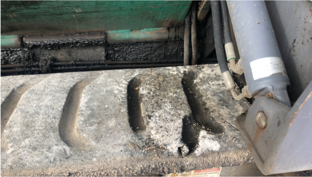
Gouge / Left Track Condition / 12-03-2020
