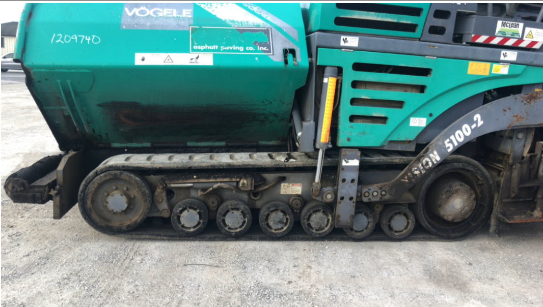
Gouge / Left Track Condition / 12-03-2020
