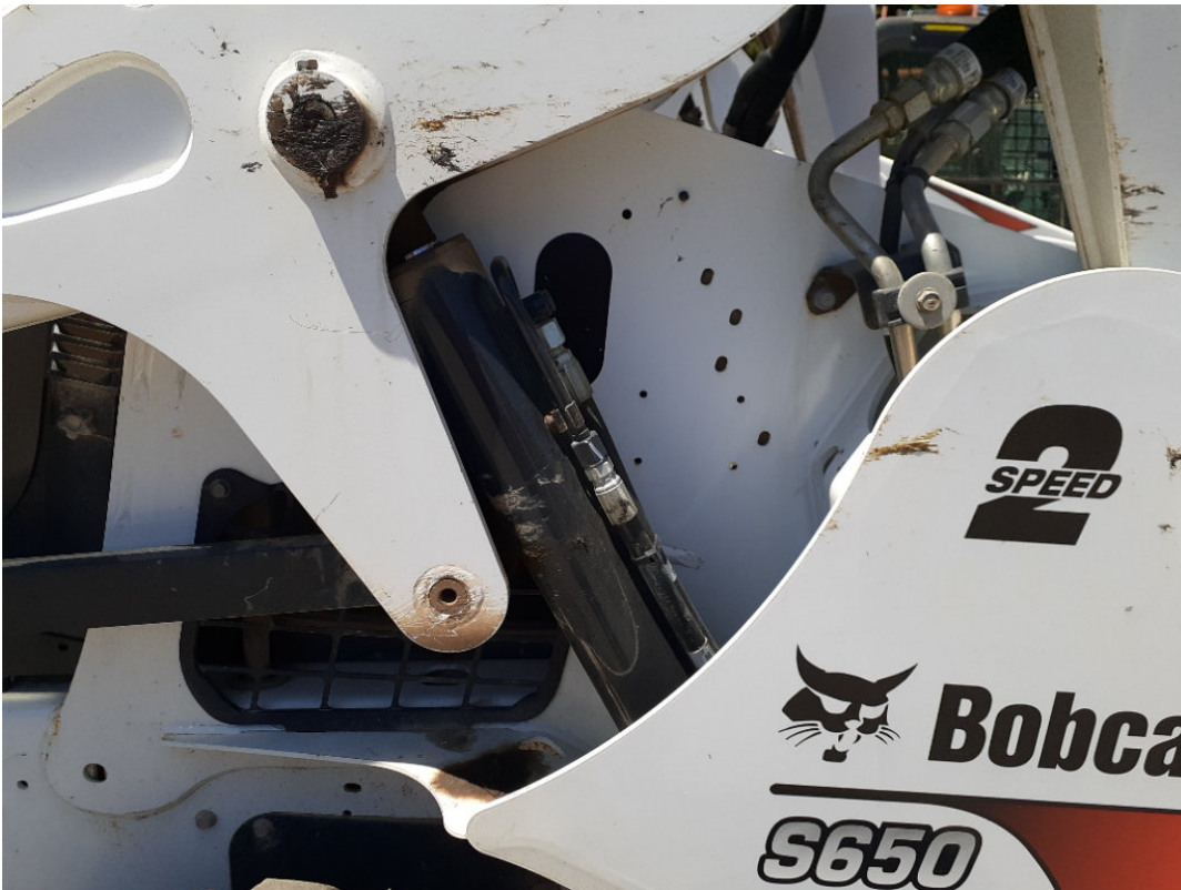
Left / Lift Cylinder / 06-18-2020
